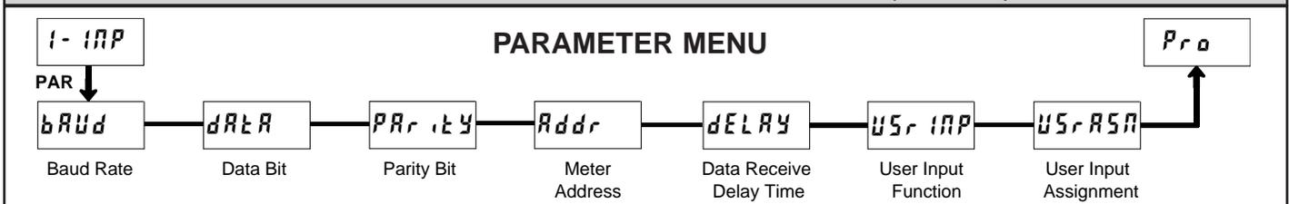
Module 1 is the programming module for the Input Setup Parameters. This includes the Serial Input setup parameters and the User Input function. Set the Serial Input parameters to match the settings of the host device.
