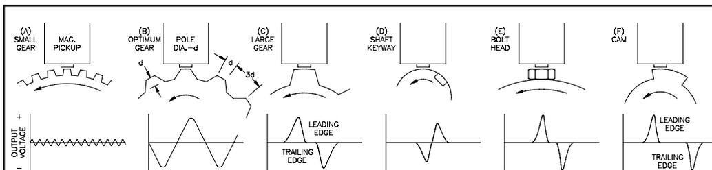
FIG. 1 OUTPUT WAVEFORMS WITH VARIOUS TARGET SHAPES & SIZES
