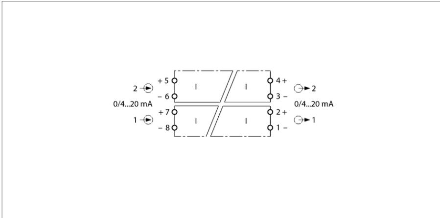
The 2-channel IMS-AI-DLI-22-DLI/L analog signal isolator is designed to transmit normalized active current signals galvanically isolated.
